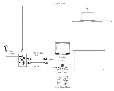
Figure 5. Complete installation
